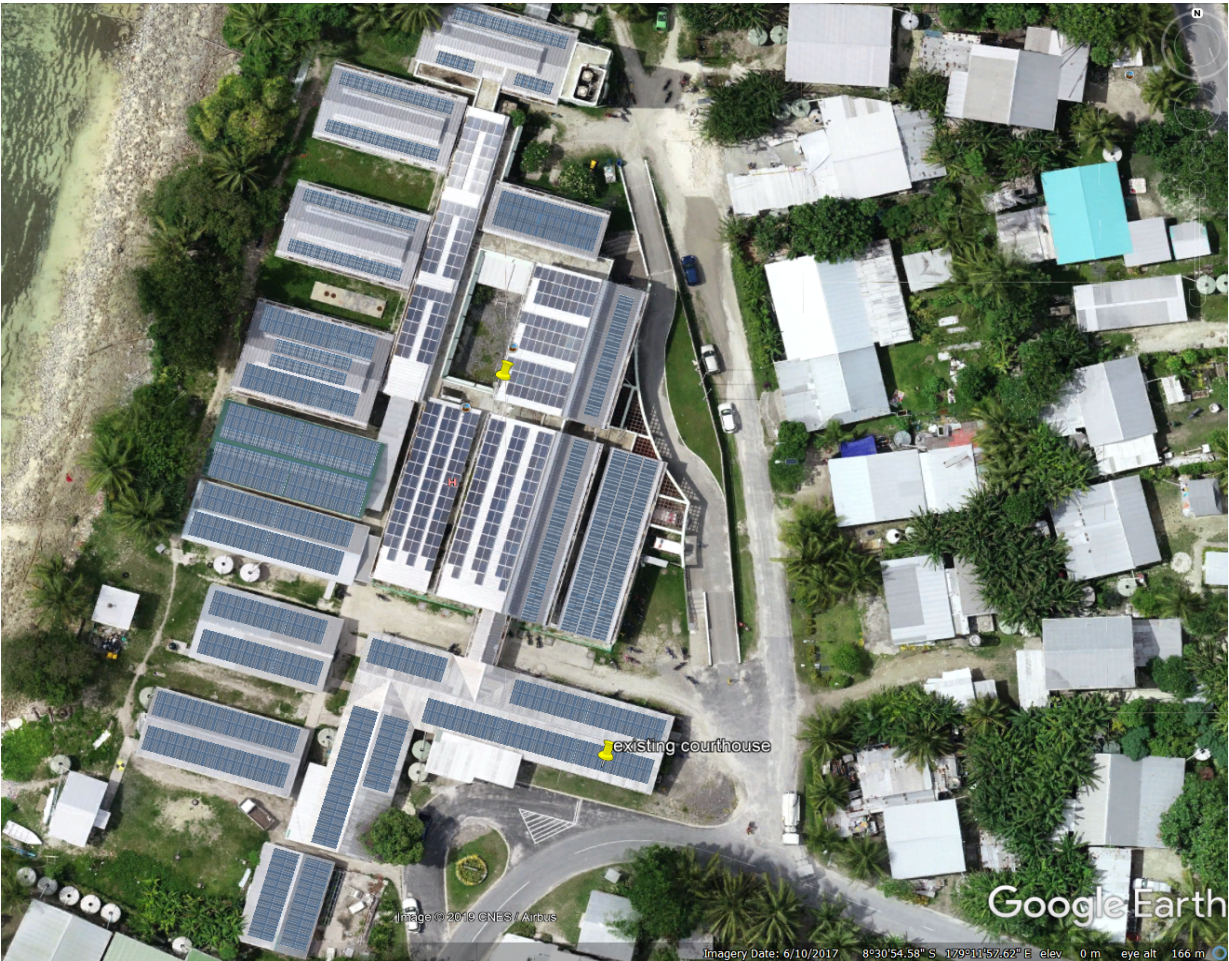
Figure B.9: The Hospital rooftop aerial view, with some existing solar visible (darker blue) and proposed solar over-laid (lighter blue).
