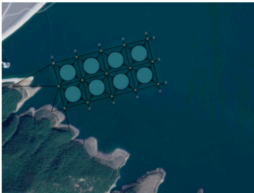
Figure 7.5: A concept plan view of the Ocean Sun mooring arrangement. sourced from their website 16
